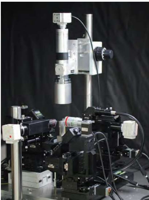
Viewing system combines our viewing units with motion control stages.
